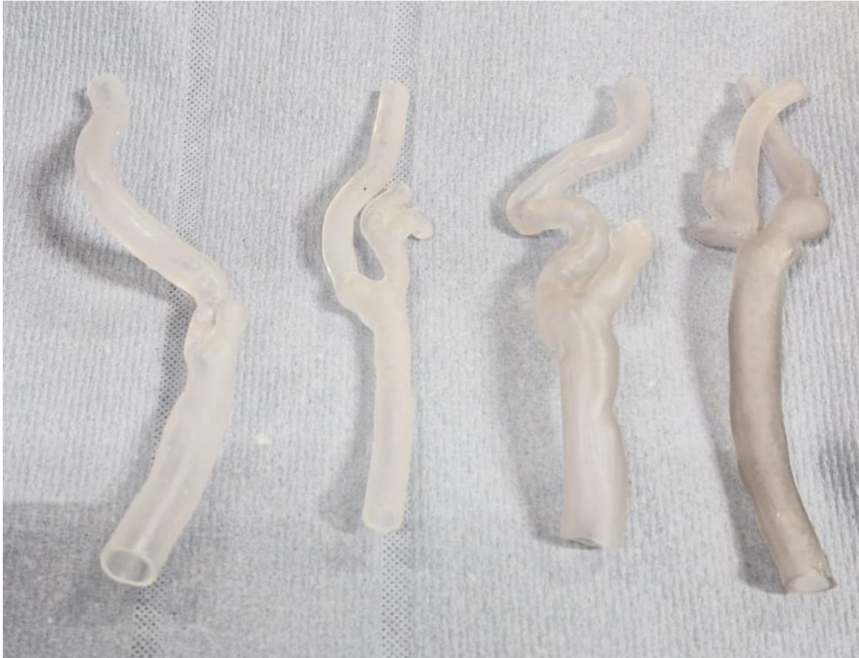
Figure 22. Prints made of Biomed Elastic 50A V1 resin after post-processing.
