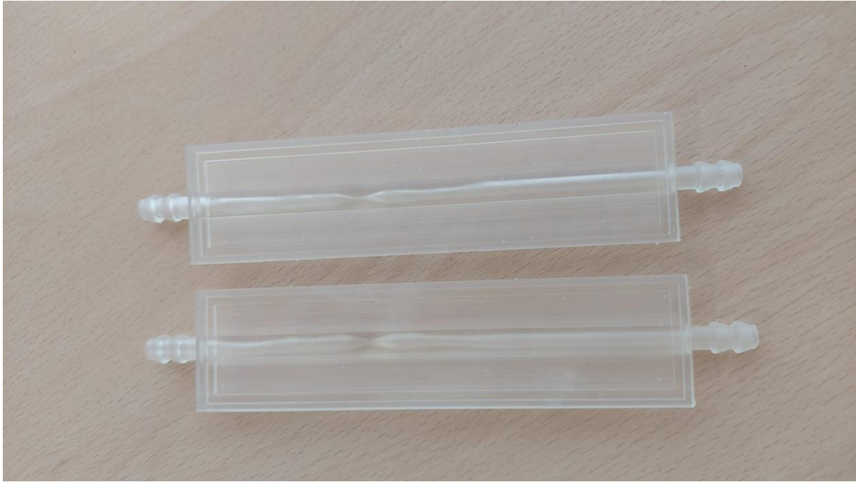
Figure 20. Clear V4 resin print for PIV measurements.
