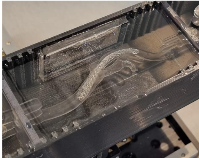
Figure 28. Experimental setup for percutaneous carotid artery stenting procedure. [P5]
